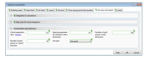
calculating the size of effect zones for flammable and toxic effects and in preparing dispersion results for plotting on Graphs. These calculations obtain the concentrations at the points on a four-dimensional grid where the dimensions are x location, y location, z location and time. The same grid is used in the post-processing that is performed for continuous observers.
