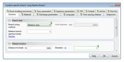
and the **Hole diameter** field is displaying a value of 224.4 mm because a circular hole with this diameter has an area twice that of the pipeline cross-section. If the breach were at the end of the pipeline, the **Hole diameter** field would show a value of 158.7 mm.
