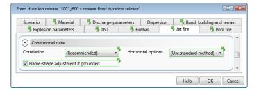
If the option is checked, adjustments are made to the angle and/or elevation of the cone so that it does not impinge on the ground, and this adjusted flame is the flame used in radiation and effect calculations.
