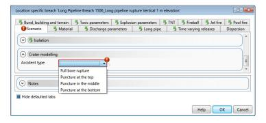
The *Puncture* options involve simple holes, whereas the *Full bore rupture* is a breach that propagates along the pipeline for a distance set by the **Fracture length**, which is a new field in the Long pipe tab section for both types of Breach Scenario. The **Fracture length** field is supplied with a default value that is set in the Long pipe tab of the Discharge Parameters; the default value supplied with the program is 10 m, which is a typical distance between couplings in a long pipeline.
